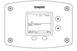
6. Differential (Display only - shows the differential of the thermostat)
